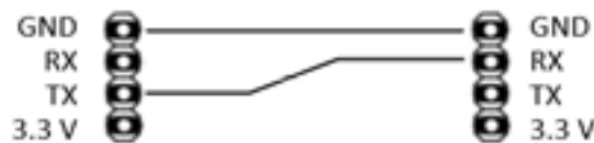
Figure 2. Cross-connect UART of two controllers. Leading controller is on the left and driven on the right
